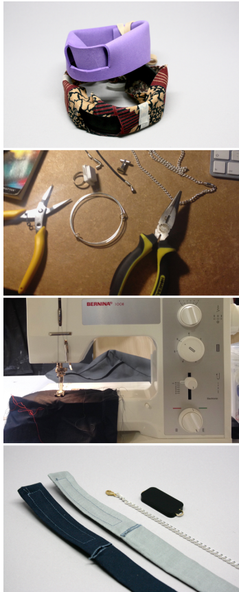
Figure 3: P6's design and the making of the prototype using sewed materials, 3d printed elements and jewellery making components.
