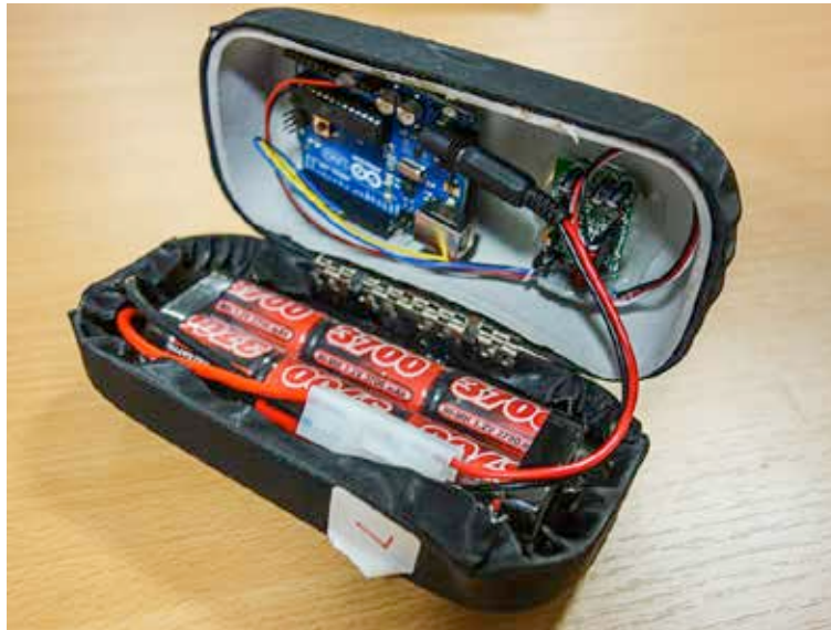
Figure 4.5.3 ActivityCounter with battery installed
