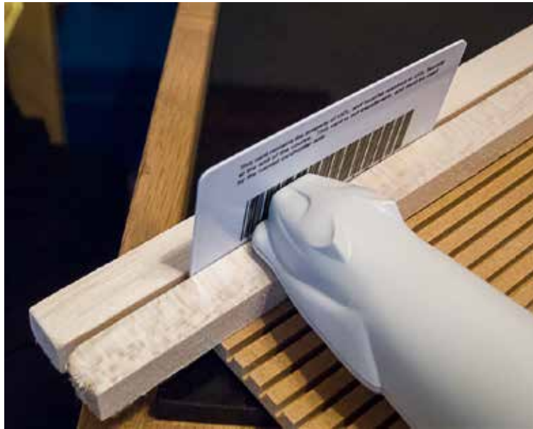
Figure 5.2.2 Prototype of a slot for scanning barcodes with a CueCat
