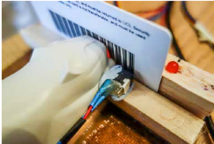
Figure 5.6.2 Switch to detect card in slot
