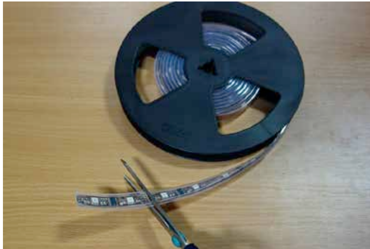
Figure 3.2.3 LPD8806 LED Strip
