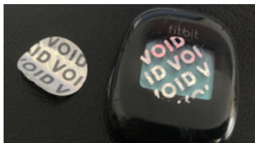
Figure 3.6 – Fitbit with tamper evident sticker removed
