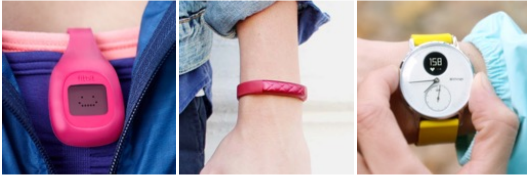
Figure 2.5 – Activity trackers in different form factors. (from left to right) Fitbit Zip clip 9 , Jawbone UP3 wristband 10 , Withings Steel HR watch 11
